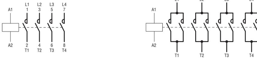
**CONTACTORES TETRAPOLARES EN DC (AC/DC para BF40E...BF150E)**
